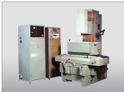
Figure 9.8. Electro-discharge jig-copying machine produced by Joint stock company "Kauno stakles" (Lithuania)
