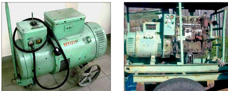
Figure 9.11. Welding equipment produced in Vilnius Electrical Welding Equipment factory: electric motor and engine driven welding machine
