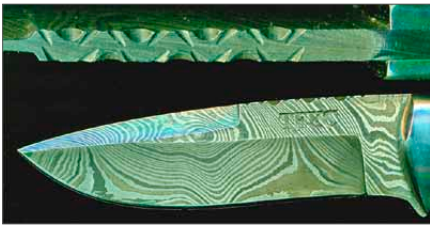
Figure 9.9. A typical smithy (a) and pattern welded knife blade (b)
