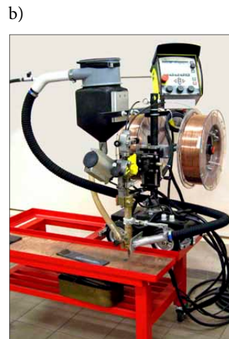
Figure 9.14. Submerged arc welding: a – scheme for the welding process; b – modern SAW equipment
