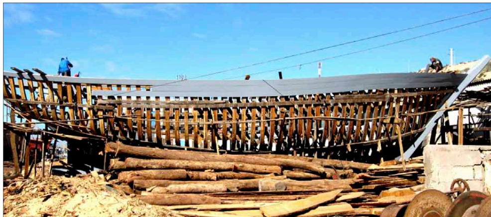
Figure 2.8. The yard of fishing in Agadir (Marroco). The boats are about 15 m in length and all hand built from eucalyptus as they have been for centuries
