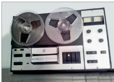
Figure 11.7. Tape recorder Elfa 201 Stereo manufactured by Vilnius Electrotechnical Works (1986). Museum of Energy and Technology, Vilnius (a). Portable cassette recorder Tonika-310 Stereo manufactured by VILMA National devices factory, Vilnius (1977–1982) (b)
