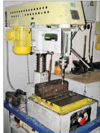
Figure 9.4. Desktop drilling machines produced in Vilnius factory "Praktika" (1979)
