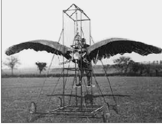
Figure 17.15. A human-powered ornithopter (1902)
