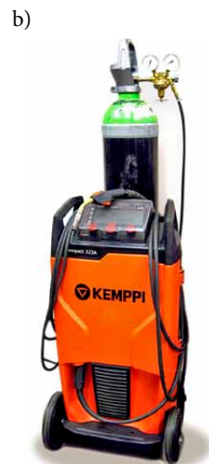
Figure 9.12. Gas metal arc welding: a – scheme for the welding process; b – modern GMAW equipment
