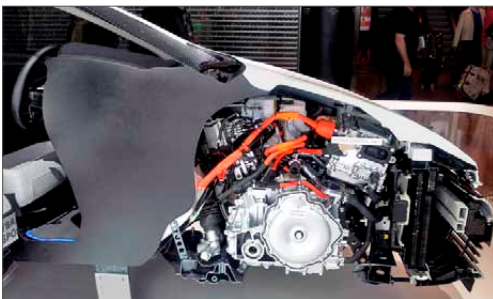
Figure 20.25. Hybrid car (Toyota) cutaway model showing engine connection and location (2013)
