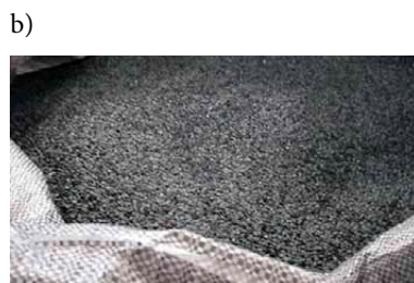
Figure 24.5. Recycling plastics: a – plastic scrap, b – converted material – PE granules
