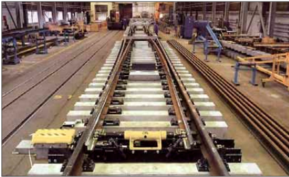
Figure 21.7. The production of straight and curved switches in the Voestalpine VAE Legetecha factory (2013)
