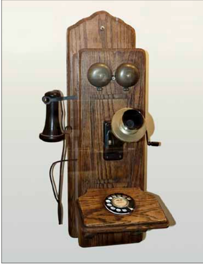
Figure 12.6. A wooden wall telephone with a hand-cranked magneto generator
