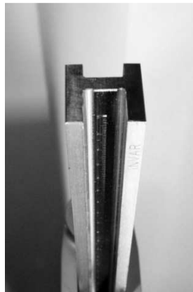
Fig. 1.17. Reference scale with 1 mm grating
