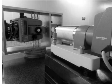
Fig. 2.10. The setup of instrumentation for the vertical angle measuring system calibration with a mirror and autocollimator
