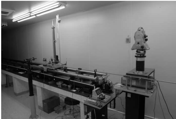
Fig. 3.1. Arrangement of the system for the calibration of vertical angle measuring systems using reference scale
