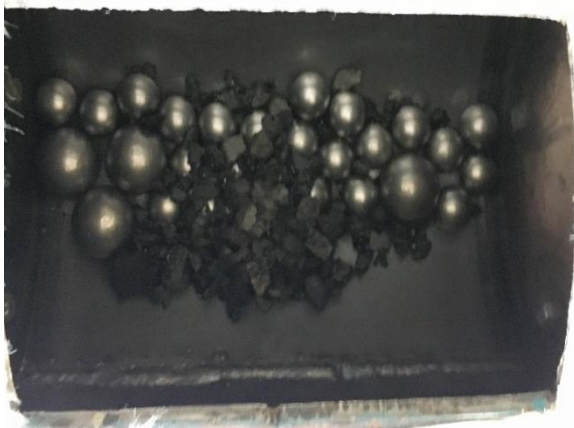
Figure 6. Industrial waste slag and balls placed in ball milling machine
