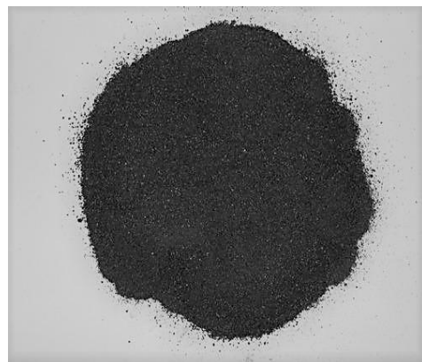
Figure 5. Industrial waste slag after ball milling and sieving
