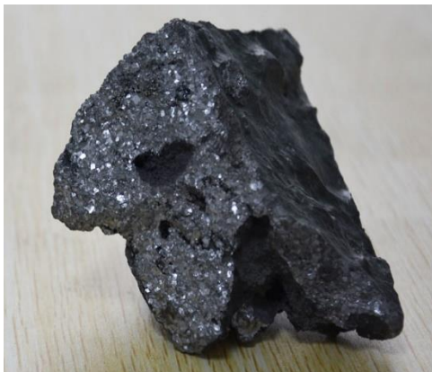
Figure 4. Industrial waste slag in raw form
