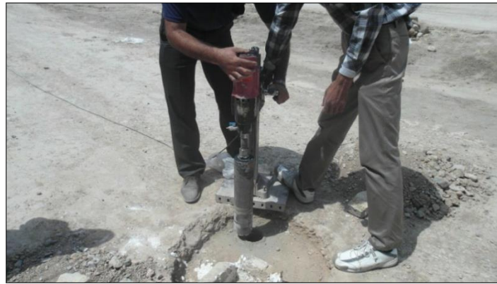
Figure 18. Sampling procedure for the uniaxial test
