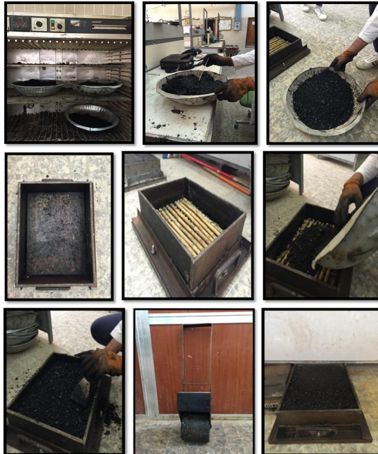
Figure 6. Slabs preparation compacted manually by hand wheel roller
