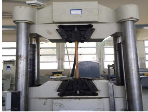
Figure 4. Tension test for reed samples
