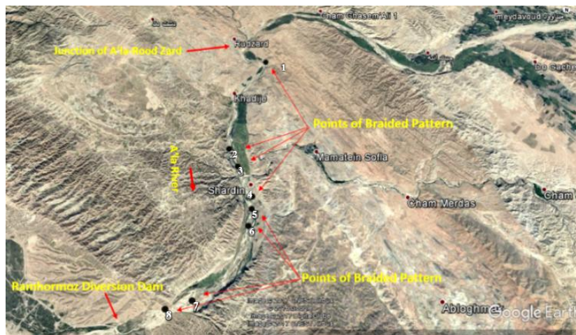
Figure 9. Braided pattern of A'la River within the studied reach of the river
