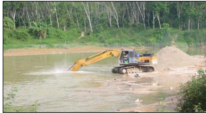
Figures 2. Aggregate mining out of riverbed by machineries
