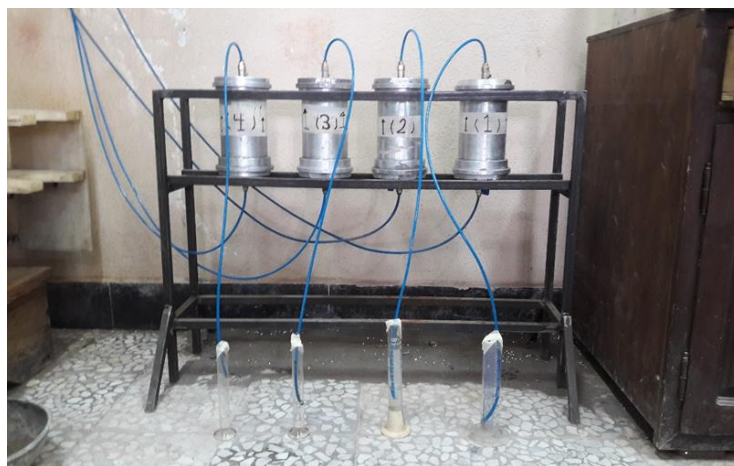
Figure 4. The test mold and inlet and outlet pipes
