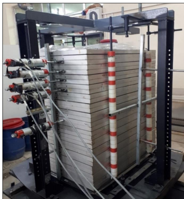
Figure 4. Laminar shear box utilized in current study
