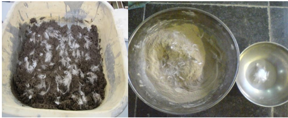
Figure 1. Addition of polypropylene fiber to a) clay-sand and b) clay mixtures
