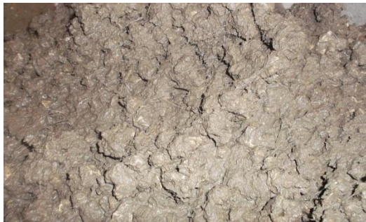
Figure 4. Fresh state of concrete when Kantharo suter fibers were added in mix
