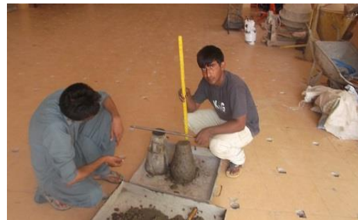
Figure 5. Slump test of fresh concrete
