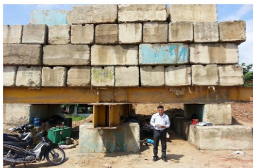
a) Static load test for group SCpile
