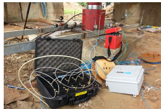
b) Equipment for load test
