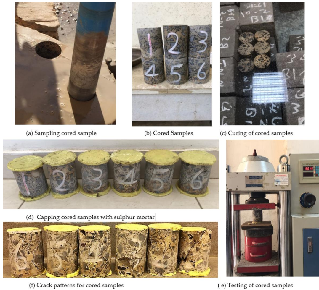
Figure 3. Cored test preparation for the demolished material
