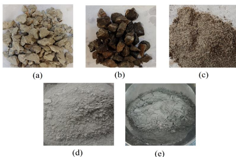
Figure 2. Overview of materials (a) RCA, (b) NCA, (c) Fine aggregate, (d) OPC, and (e) FA
