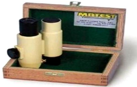
Figure 9. Micro-crack meter that used in this work
