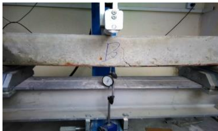
Figure 5. Concrete beam under bending test
