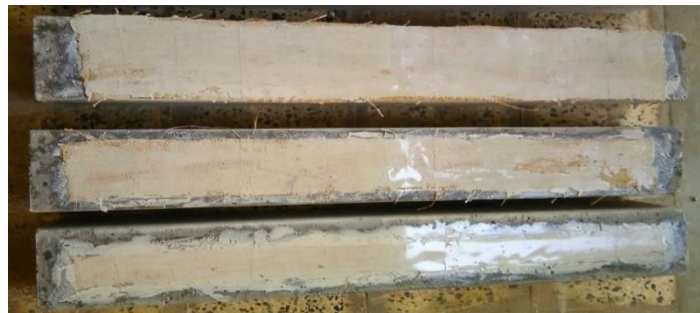
Figure 4. Strengthening beam with jute fibers
