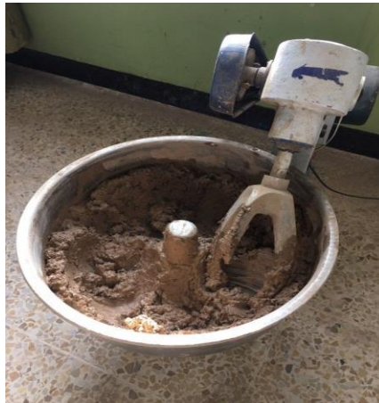
Figure 7. Soil mixing device
