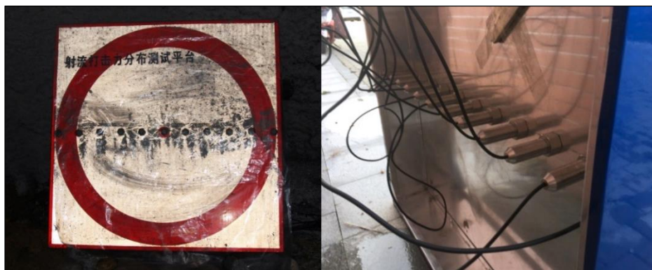
Figure 10. Assembly of the Shotcrete test platform
