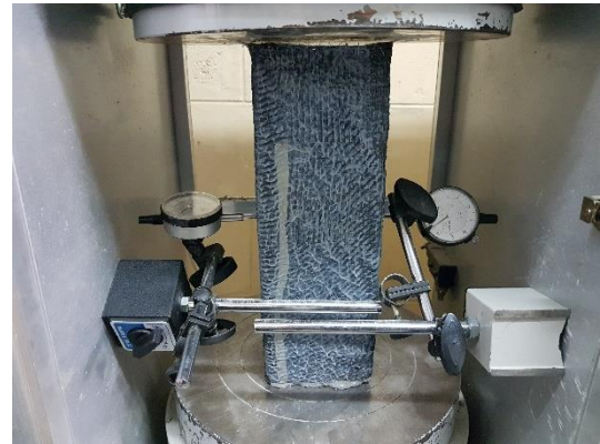
(b) Column L1-1 at failure
