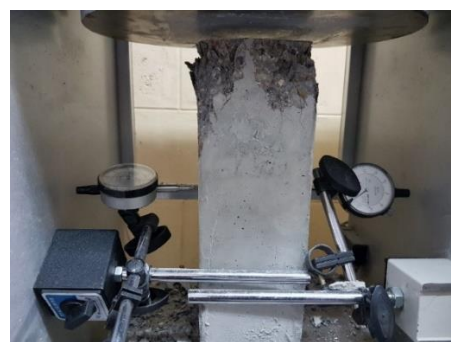
(b) Column L0-2 at failure
