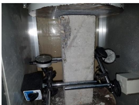
(a) Column L0-1 at failure
