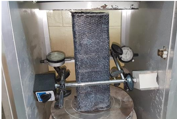
(a) Column L1-1 at failure
