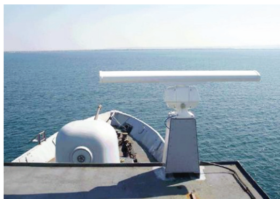
Fig 4. X-Band radar installation for wave measurement
