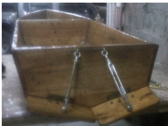
Fig 2. Flaps at the transom of the model
