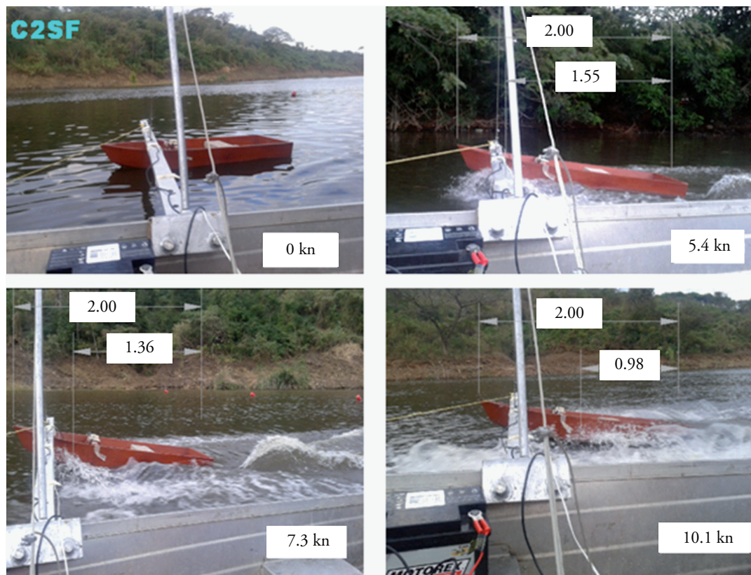
Fig. 4. Tests with no flaps in load condition 2
