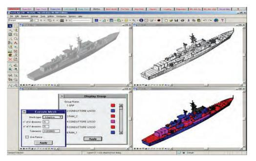
Fig 13. RCS warship analysis by Ship EDF (IDS Ingegneria dei Sistemi S.p.A.<sup>13</sup>)
