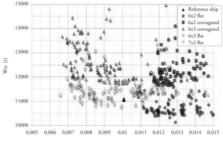
Fig 8. Outflow vs. steel weight in cargo area - Pareto designs from different configurations
