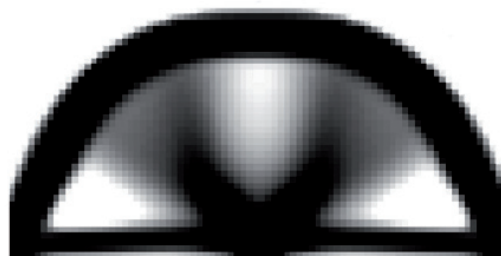
Fig. 6. Topology optimized structure with M/M_0 < 0.4
