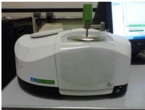
Figura 5: Espectrômetro PerkinElmer UATR Two. Figure 5: PerkinElmer Spectrometer UATR Two
