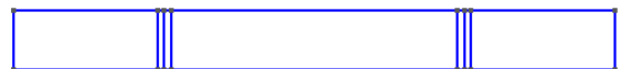
Fig. 4: Schematic of the FEM model showing the tissue and two electrodes cross-section view along the center line of the tissue
