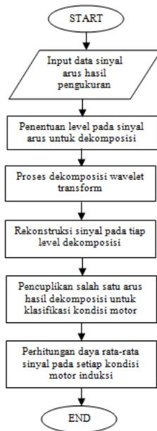
Gambar 4. Diagram alur *Decomposition Wavelet Transform*
