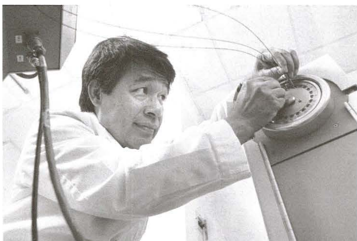
Radiation physicist Tanxia Qu, Ph.D., connects catheters to the applicators of the HDR unit, a single, high intensity radioactive source stored within a shielded safe.
