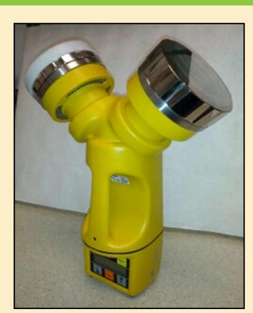
Volumetric Air Sampler
