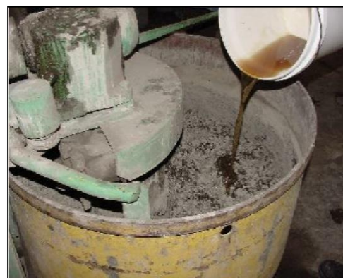
Fig- 8: Liquid component addition [19].
