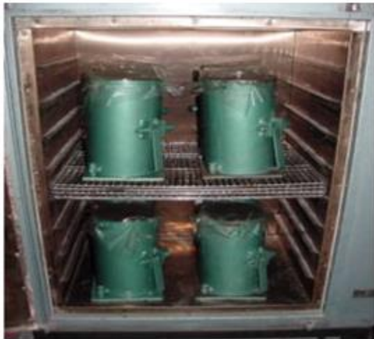
Fig -10: Dry oven curing [22]
