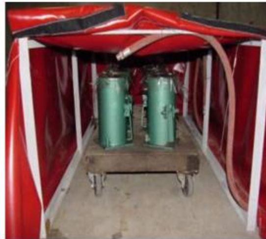
Fig -11: Steam curing [22]
