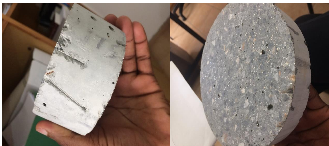
Fig-1: (a) Fibers aligned vertically on the wall of the cylinder (b) A section through the cylindrical specimen showing the cut fiber surface
