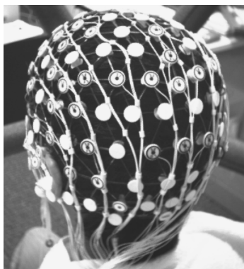
Fig. 2: A sensor net of 64ch Dense Array EEG from EGI
