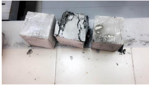
Fig 7: Compressive strength test on concrete
