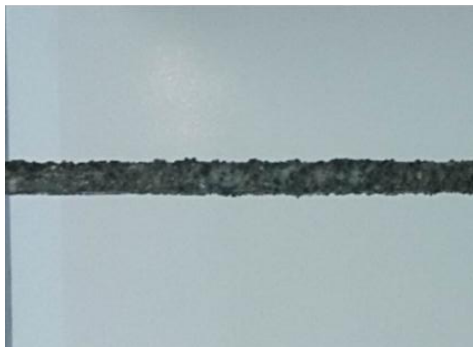
Fig 8: Sand coated GFRP bar
