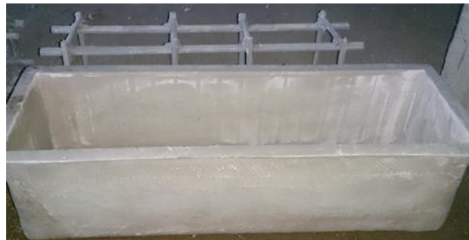
Fig 9: GFRP Formwork with rebar arrangements
