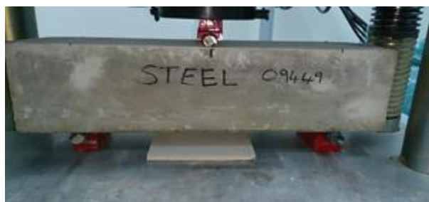
Fig 13: Flexural test on RC beam
