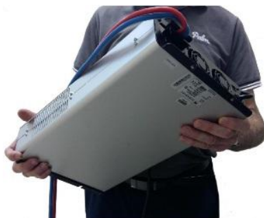
Fig. 15. Compact battery charger 4 kW, 0 – 250VDC
