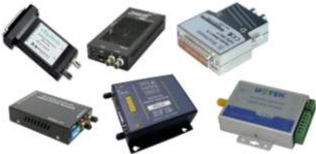
Fig. 1. Various converters of electric signals into optical, and vice versa, suitable for telecommunication systems.
