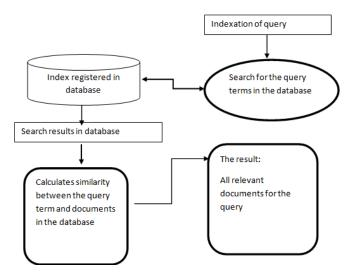
Figure. 6 The process of search in a database (db4o)
