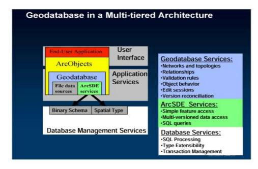
Figure 3: Geodatabase in a Multi-tiered Architecture
