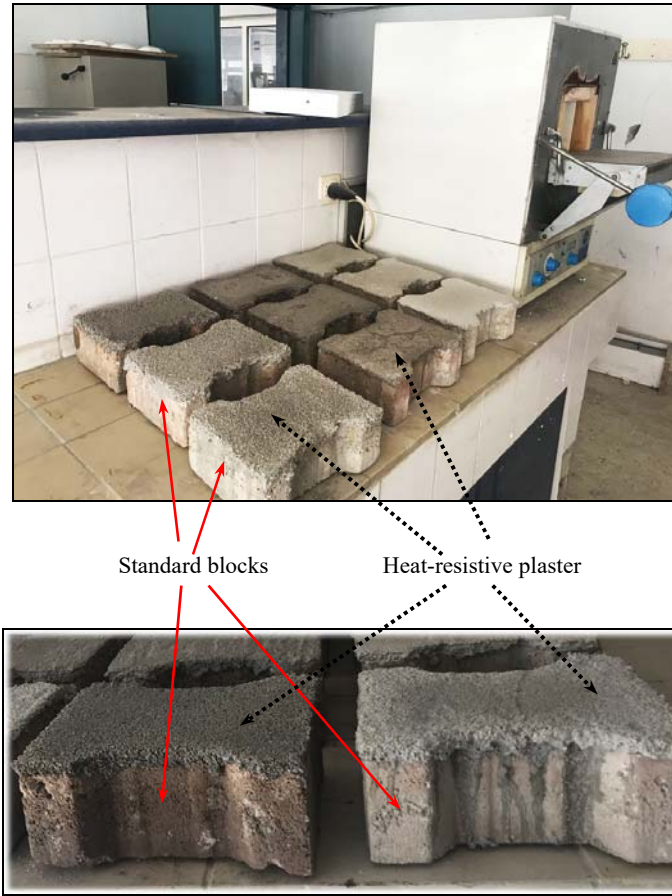
Figure 5. Heat resistant concrete pavement block samples, prepared for surface temperature tests by coating their top surfaces with especially prepared heat resistant concrete plaster.
