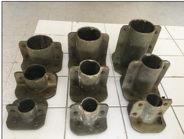
Figure 3. Molds specifically designed for bond tests.
