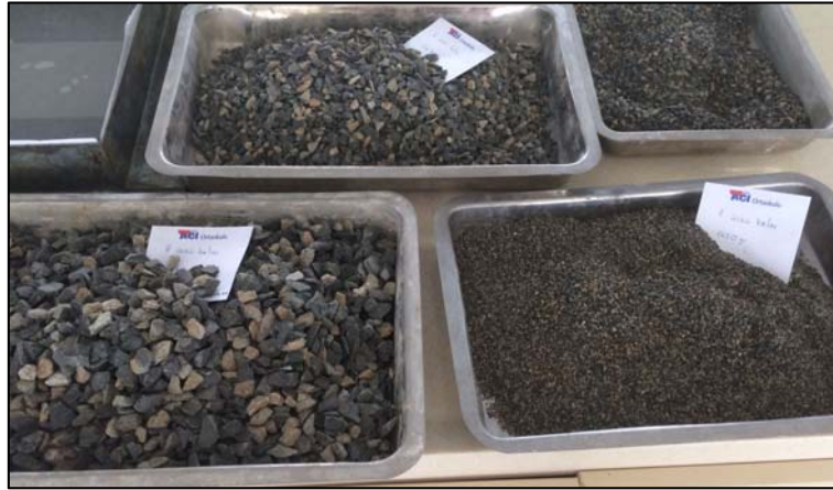
Figure 2. Basalt aggregate used in the production of concrete.
