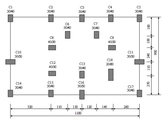
Figure 8. Ground storey floor plan of the building (dimensions are in cm)
