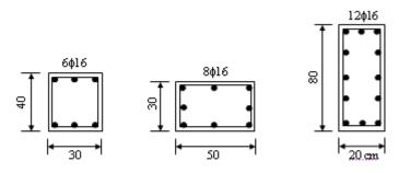
Figure 9. Dimensions of the column and rebar arrangement
