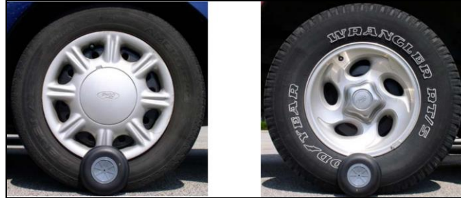
Figure 4. Comparison of scaled tires and full-scale tires [1]
