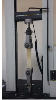
Figure 2. Testing of Cynara scolymus / PET nonwoven composite.
