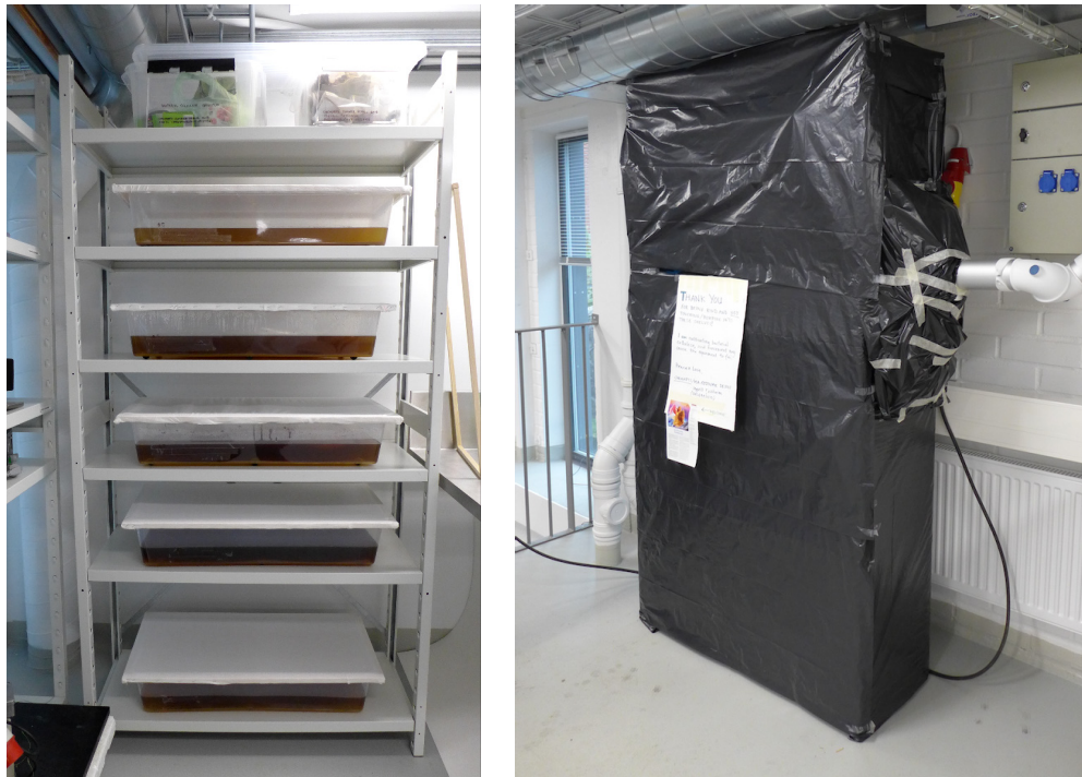
Figure 19 Microbial cellulose cultivation. First version and second version of my cultivation station. The photos show the cultivation stations with and without black covering. The main difference between the two setups was the air extraction funnel/hood connected to the second version, shown here with black plastic covering.
