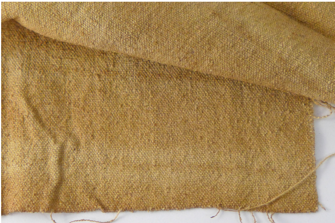
Figure 7 Dyeing experiments with chaga. Colour results from 3 days of immersion. Both fabrics are silks. The texture on the upper fabric is caused by a synthetic substance I treated the material with before the dyeing. The texture on the lower fabric is due to the chaga colourant. The colouring and pigmentations was embraced as a feature of the designed costumes, emphasising folds and structure in the fabric. This sense of tracing, of handled material and time, added another layer of narrative to the costume garments.
