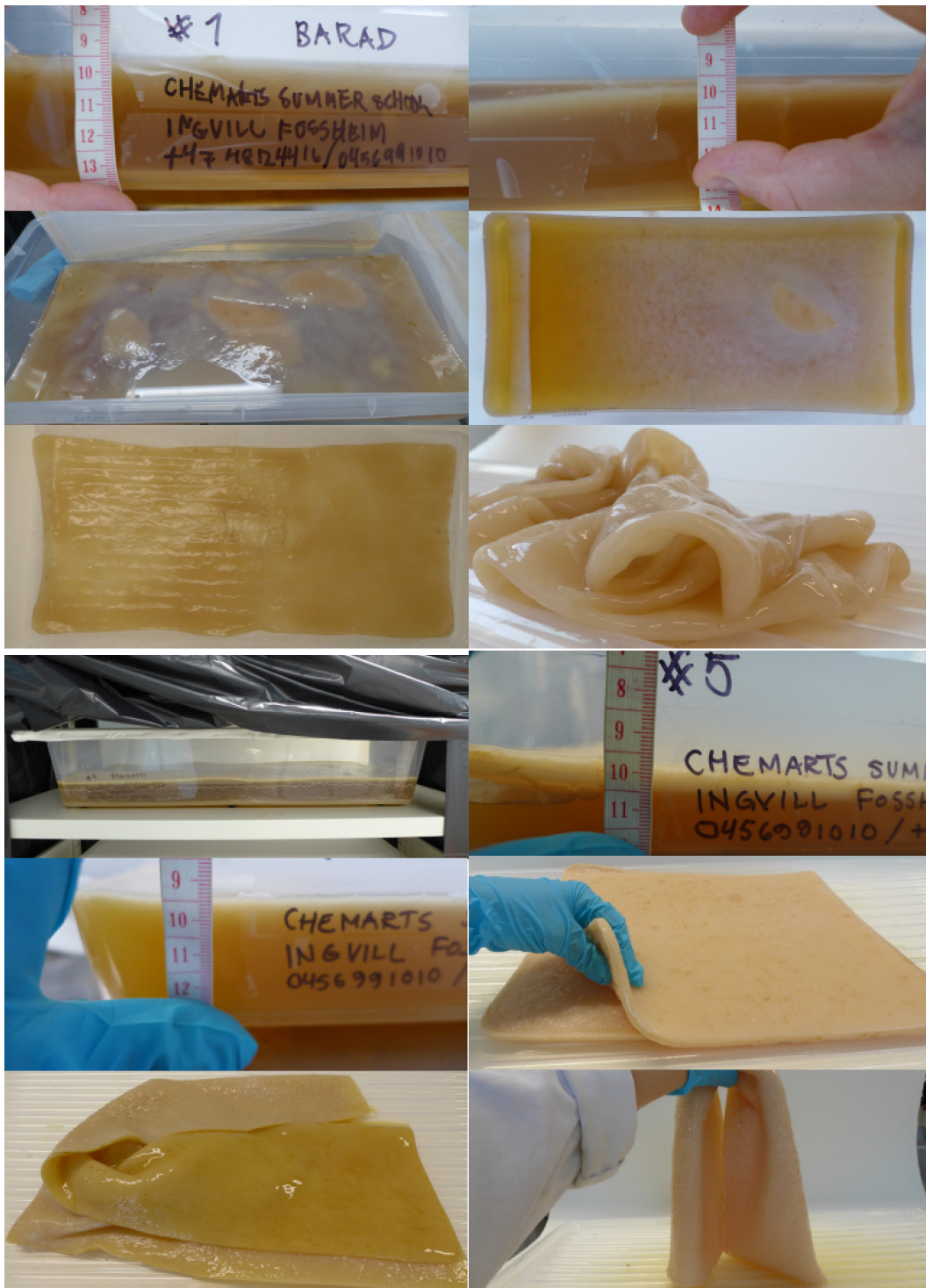
Figure 21 Microbial cellulose cultivation. The photographs document thickness of the wet microbial cellulose, and its appearance just before and just after harvest and disinfection, after approximately five weeks of cultivation.
