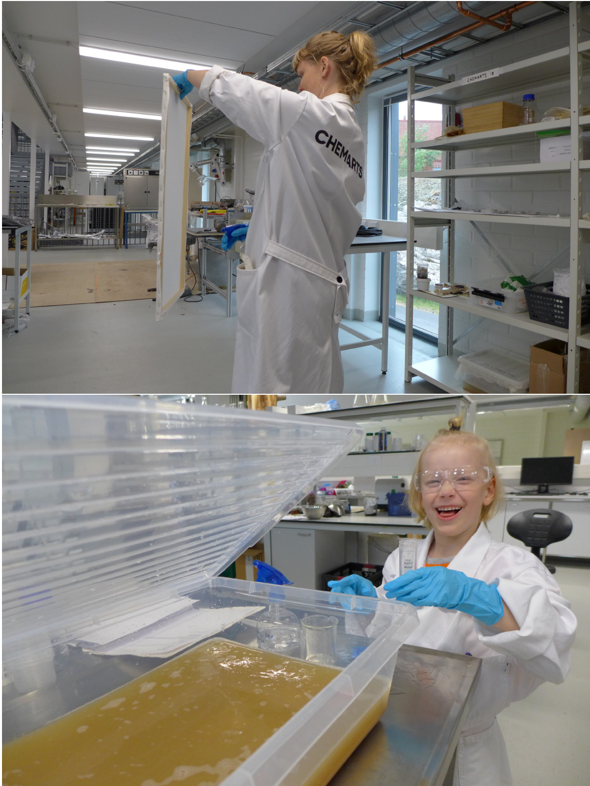
Figure 20 Microbial cellulose cultivation. Upper image: Disinfecting the custom made, breathable lids for the containers, photo by Alvar Salminen Fossheim. Lower image: a smelly G. xylinus is transferred from laboratory storage container into the cultivation medium with the aid of my assistant.
