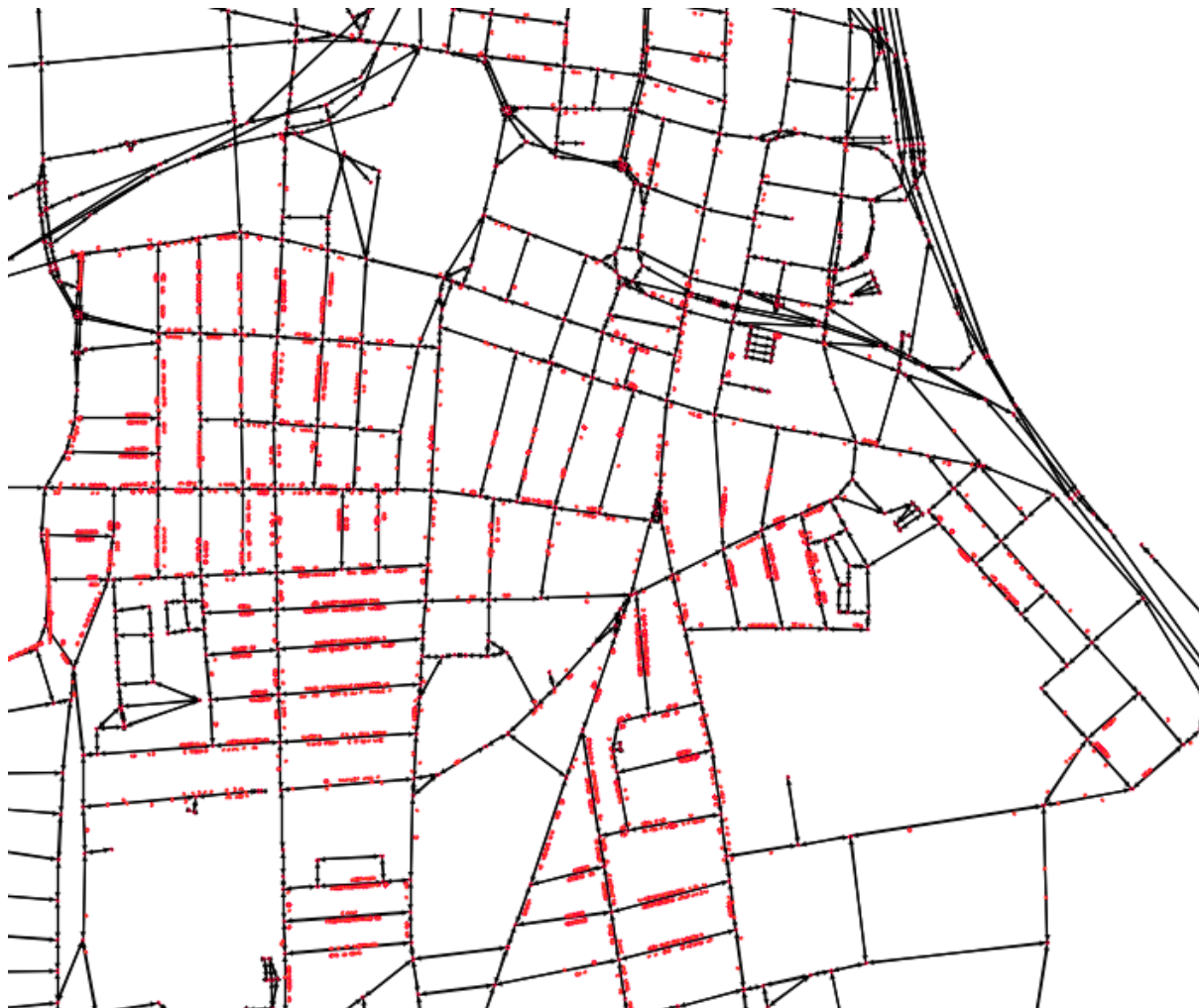
Figure 4: (Color online) A view of a portion of the actual street network with meter locations in the UTM format serviced by Connecticut Natural Gas in our data set from Hartford, Connecticut. The red dots represent the meters. This network is used for our simulation experiments.
