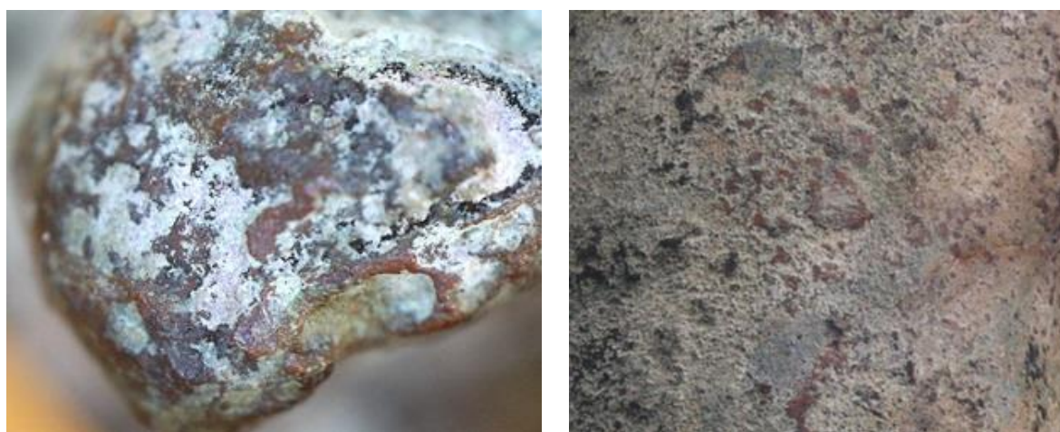
Figure 6.4: Comparison between the surface corrosion on Wadjet-Bast’s tang (A) and exfoliating scale of copper oxides encountered on the Large Cat (B).
