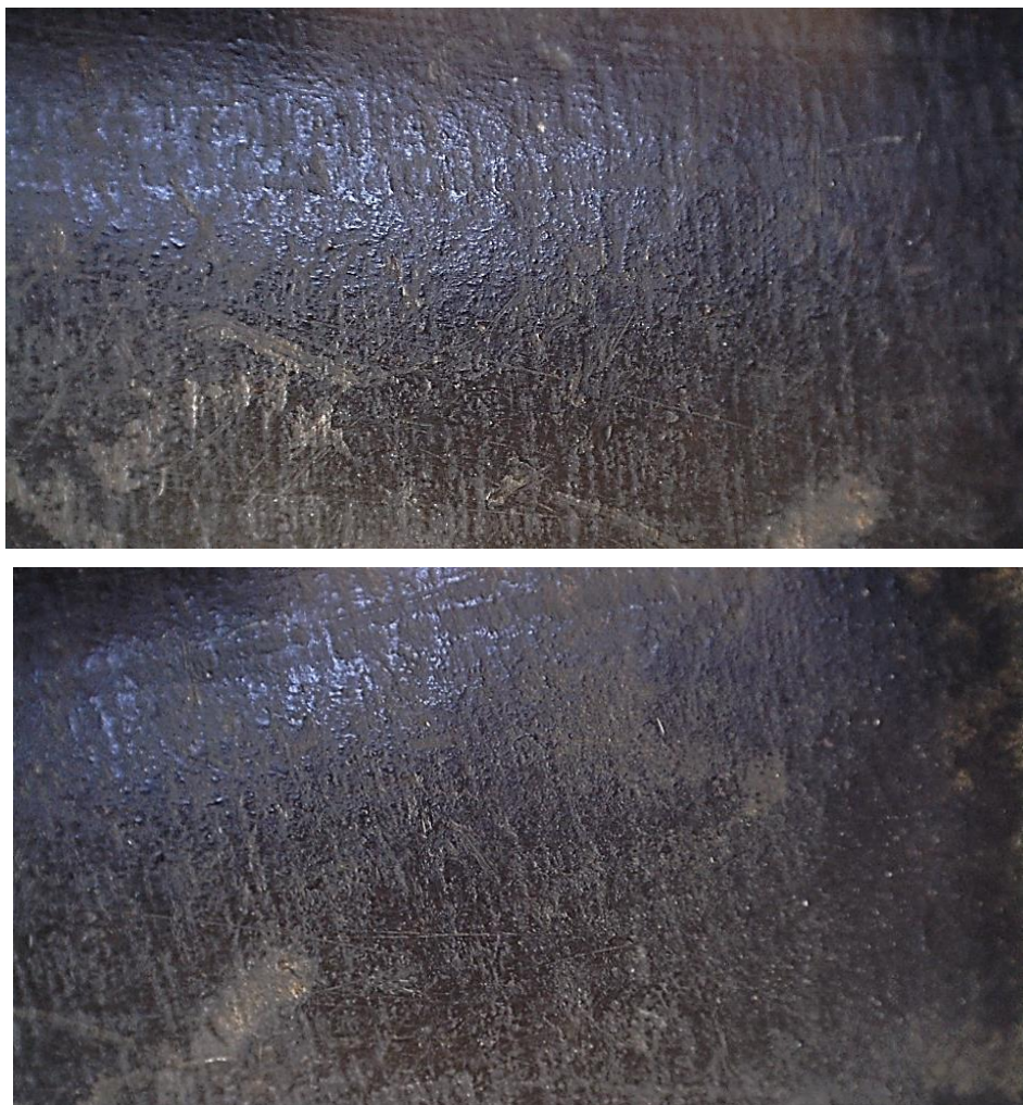
Figure 6.34: Polishing striations across the width of the Tower of London gauntlet.
