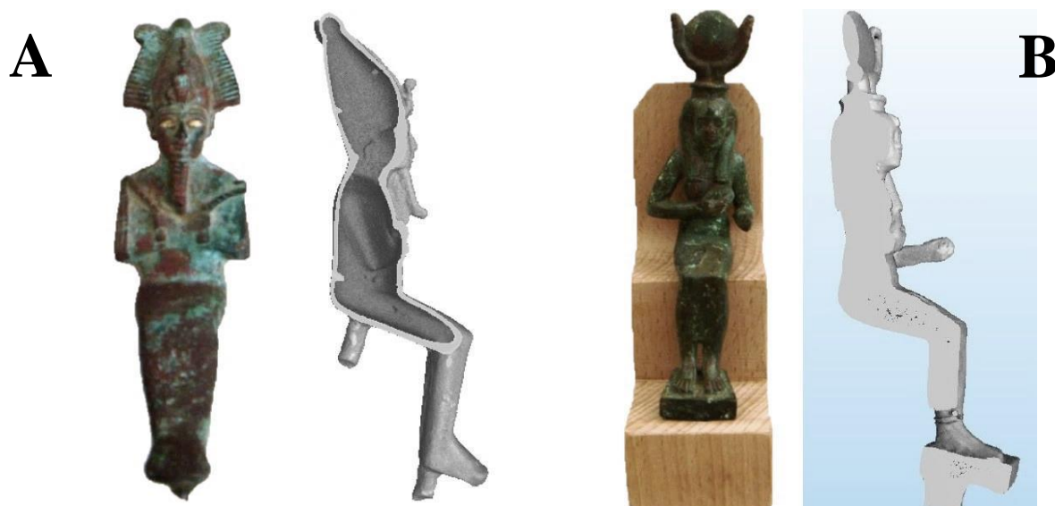
Figure 3.26: Seated Osiris figure (left) and neutron radiography (right) showing chaplets (A). Nursing Isis (left) and neutron radiography showing solid casting (B). Source: Gravette (2011, 4, 5).
