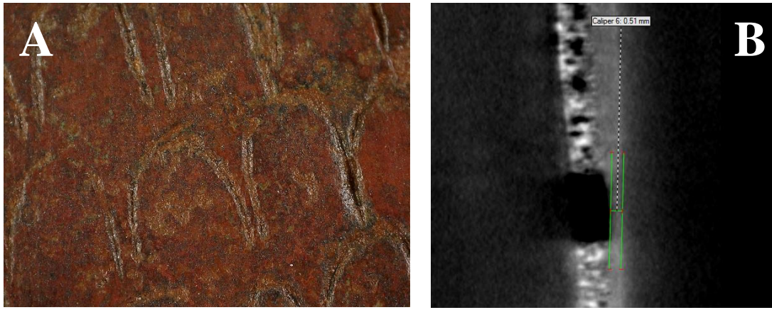
Figure 7.19: The right side of Wadjet-Bast's throne by means of digital microscopy (A) and a thin (0.51 mm) layer of bronze covering a casting hole (B).
