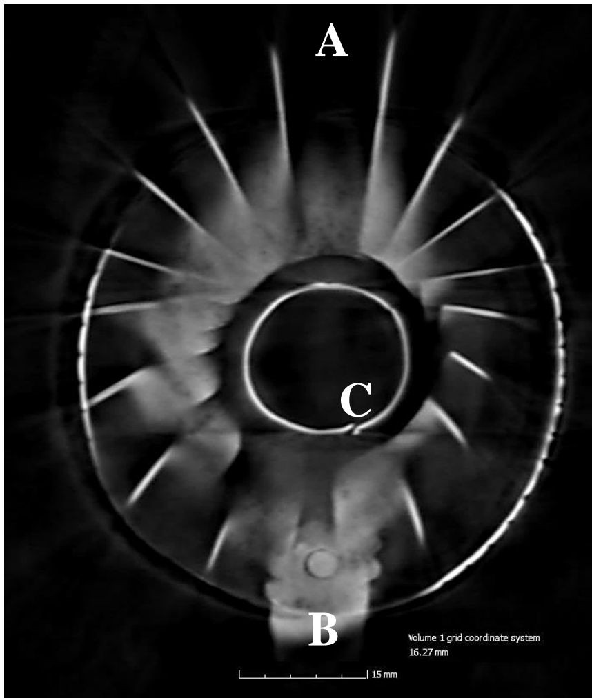
Figure 7.25: Shape of the grommet inside the tehen kanomono . The tube itself was constructed from a flat metal plate that was bent into shape. The opposite/joining edges are clearly visible (C). (A) indicates the front of the kabuto , while (B) indicates the back.
