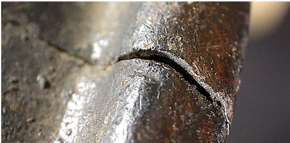
Figure 6.44: A crack along the distal edge of the Tower of London gauntlet.
