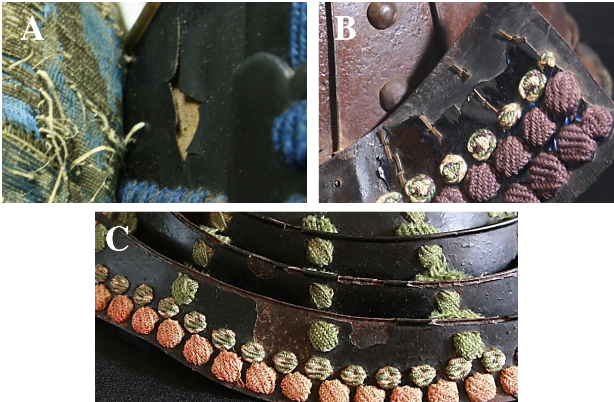
Figure 5.18: Lacquer flaking patters on the dou (A), the kabuto (B) and the menpó (C).
