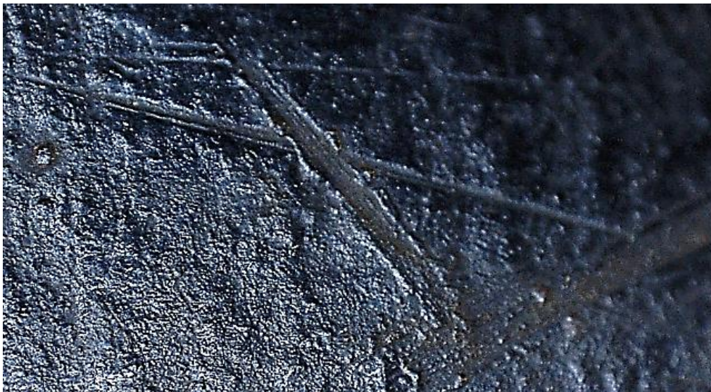
Figure 6.36: Impressions on the metal surface of the Tower of London gauntlet. The impressions appear as if an object cut across the surface while the metal was still warm and malleable.
