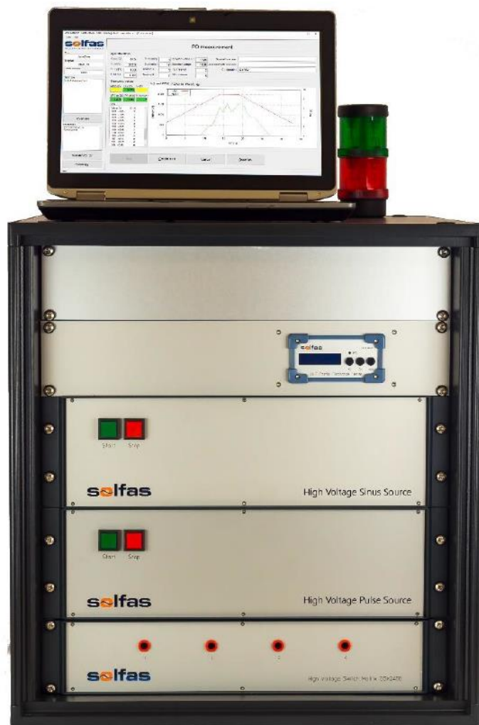
Figure 2.33. Partial discharges testbench by Solfas Technologie GmbH
