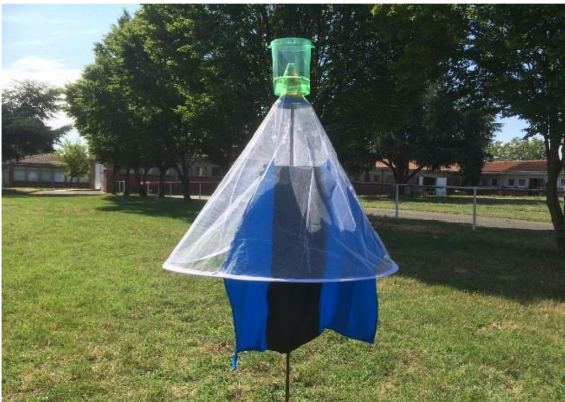
Figure 6: piège Nzi (photo originale)
