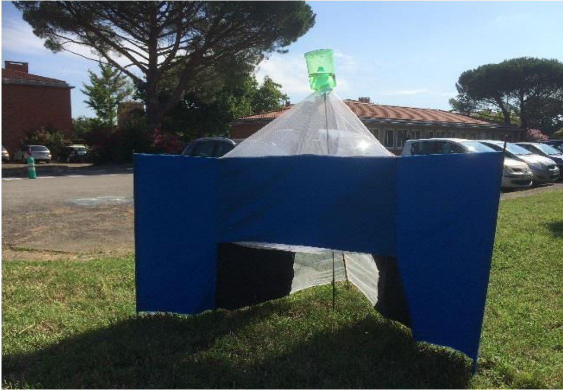
Figure 6: piège Nzi (photo originale)
