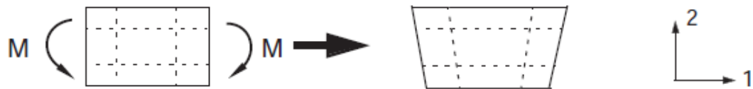
Figure 15. Deformation of 2D linear element with full integration under bending moment M [110]
