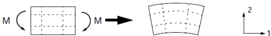
Figure 16. Ideal deformation of material under bending moment M [110]
