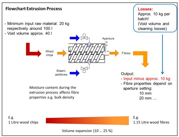
Figure 6. Flowchart showing inputs and outputs of the extrusion process at the ATB pilot plant. (Source: ATB)
