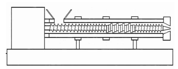
Figure 3 Single screw extruder. (Mehuys 2004)
