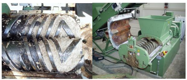
Figure 2. Open twin screw extruder with material inside (left), whole extruder opened (right). (Source ATB.)
