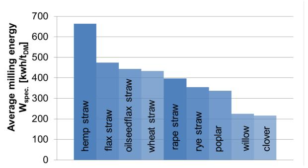
Figure 7 Average milling energy consumed by the extruder in kWh/ $t_{DM}$  at moisture content of approx. 40 % for various types of input material (Source: ATB)
