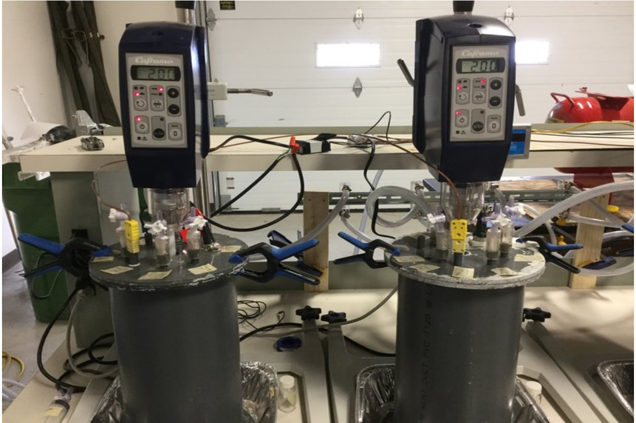
Figure 2-1: Bioreactor set-up for pilot project using Ecuadorian Tailings (ECT) starting materials.
