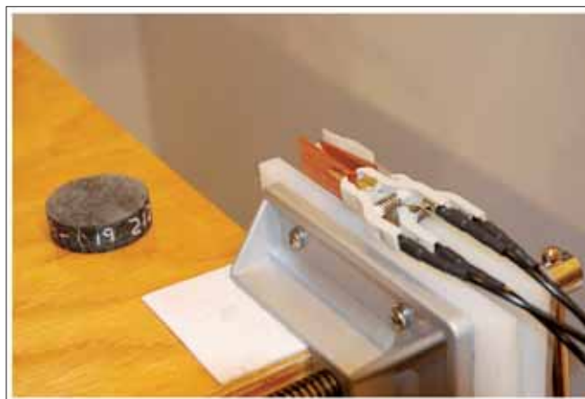
Figure 3. Apparatus (vise with plastic face plates) for clamping the sample (observed) between the copper mesh electrodes. Another sample is shown on the table. Note that the samples must be sawn with a rock saw to ensure they are flat. There is no need for polishing if the saw cut is clean.
