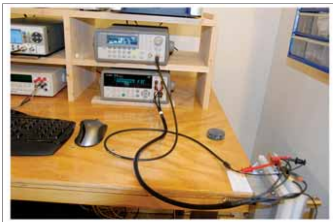
Figure 4. Signal generator and digital multimeter set up to measure the IP effects of a sample. A bipolar pulse with a period of 8 s is imposed on the sample, and voltage read at 30 or 60 samples per second for ten or more stacks.
