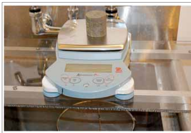
Figure 1. Balance used to measure density. Note that the scale is suspended above a sink.
